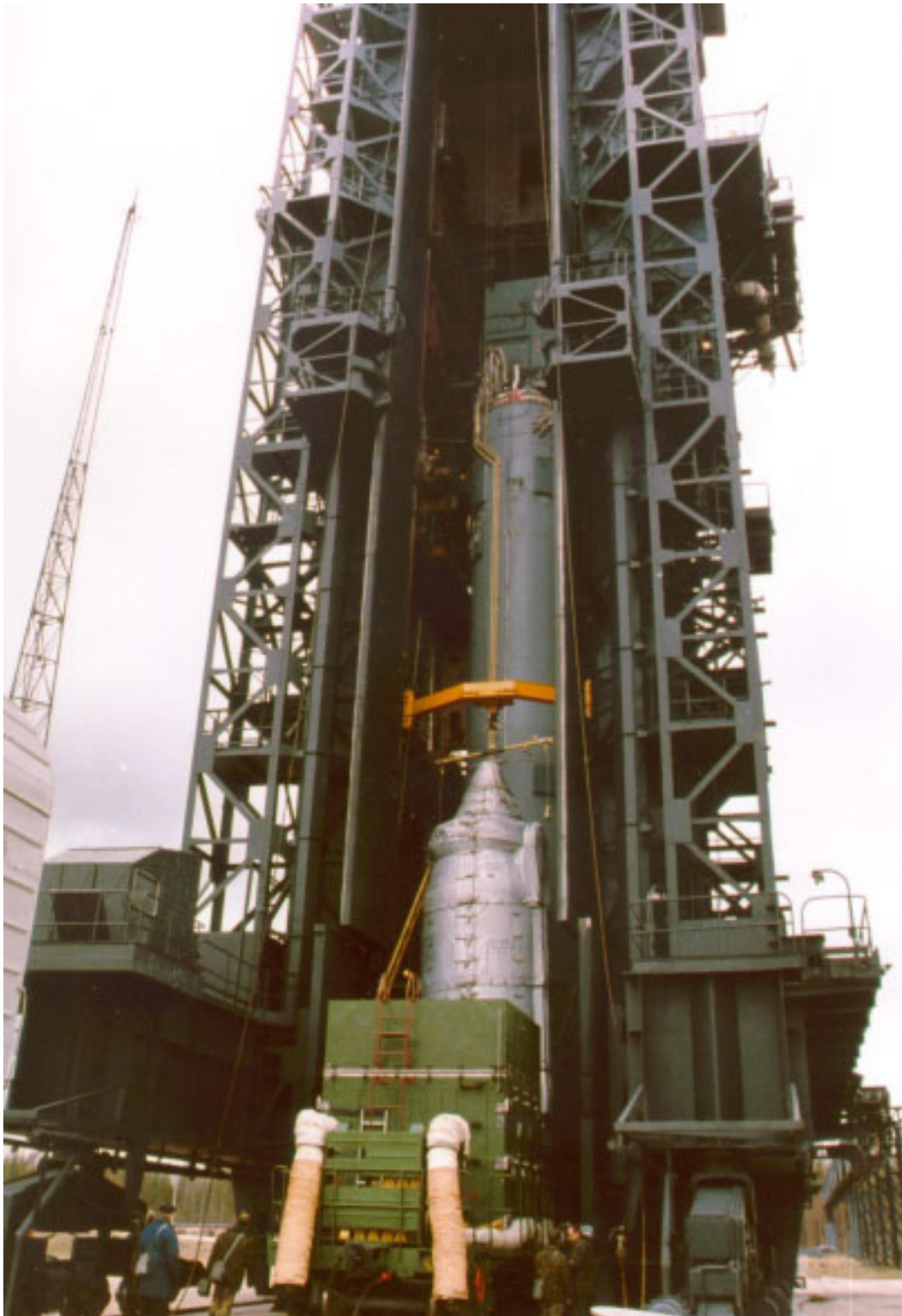
Figure 1-21: Beginning of Operations for Mating the Upper Composite with the Rockot Booster Stage (SS-19)
