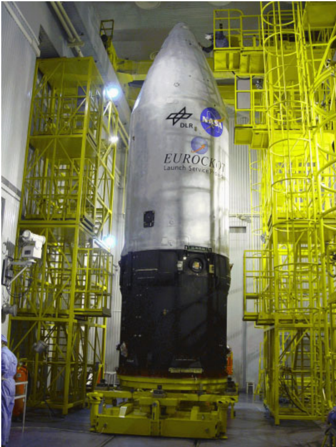
Figure 1-17: Completion of GRACE Payload Encapsulation in EUROCKOT's Payload Processing Facility
