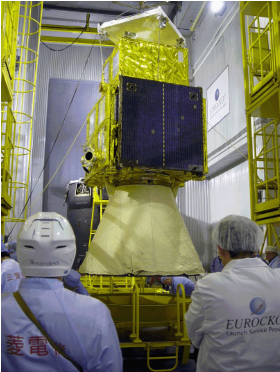
Figure 1-14: Transfer of SERVIS-1 Spacecraft for Mating Operations with Breeze-KM
