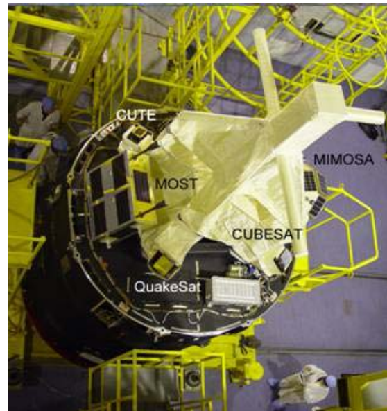
Figure 4-3: Integrated MOM Payload with Main Payload Simulator
