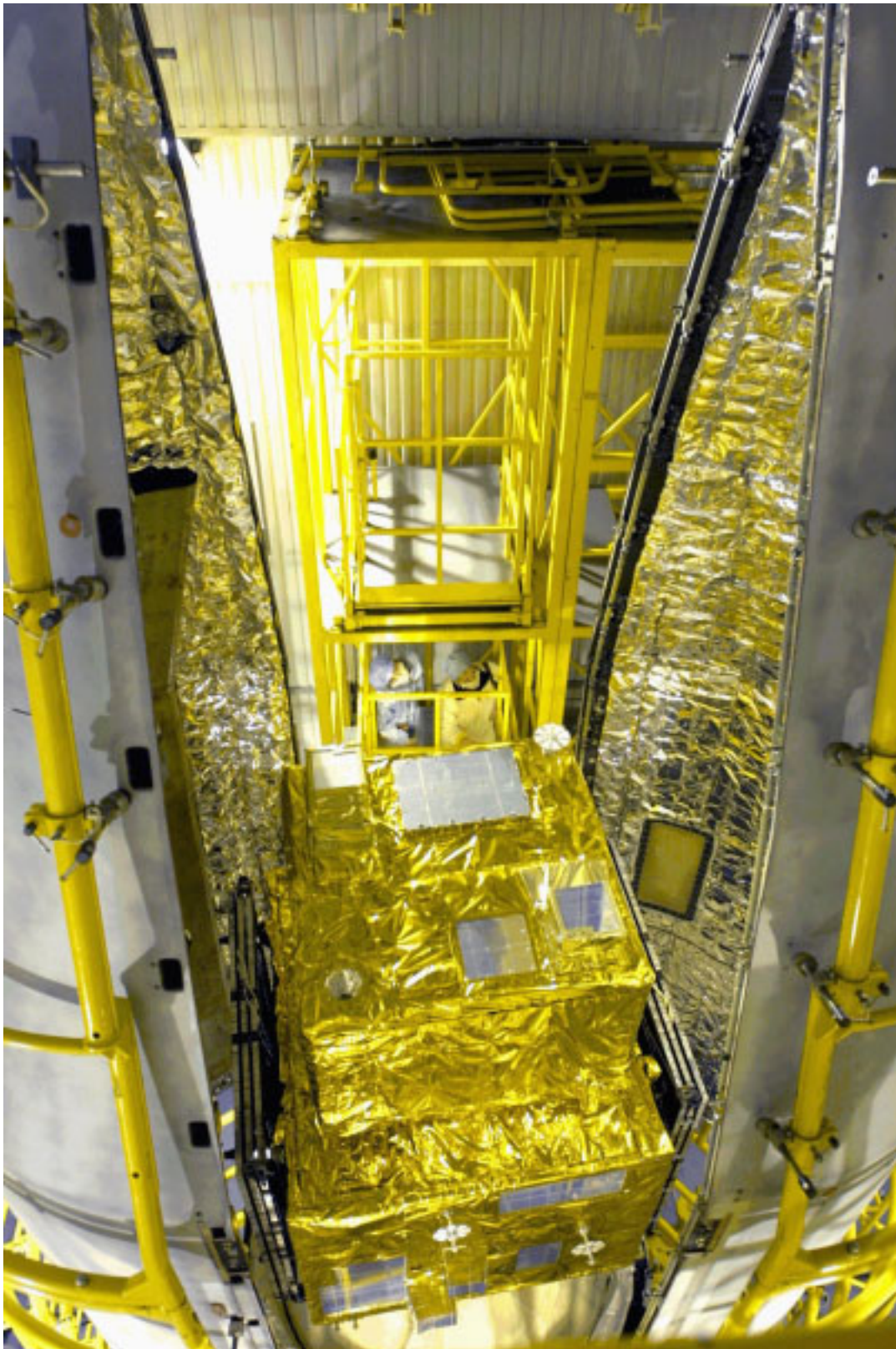
Figure 1-16: Final Encapsulation Operations of SERVIS-1 Spacecraft
