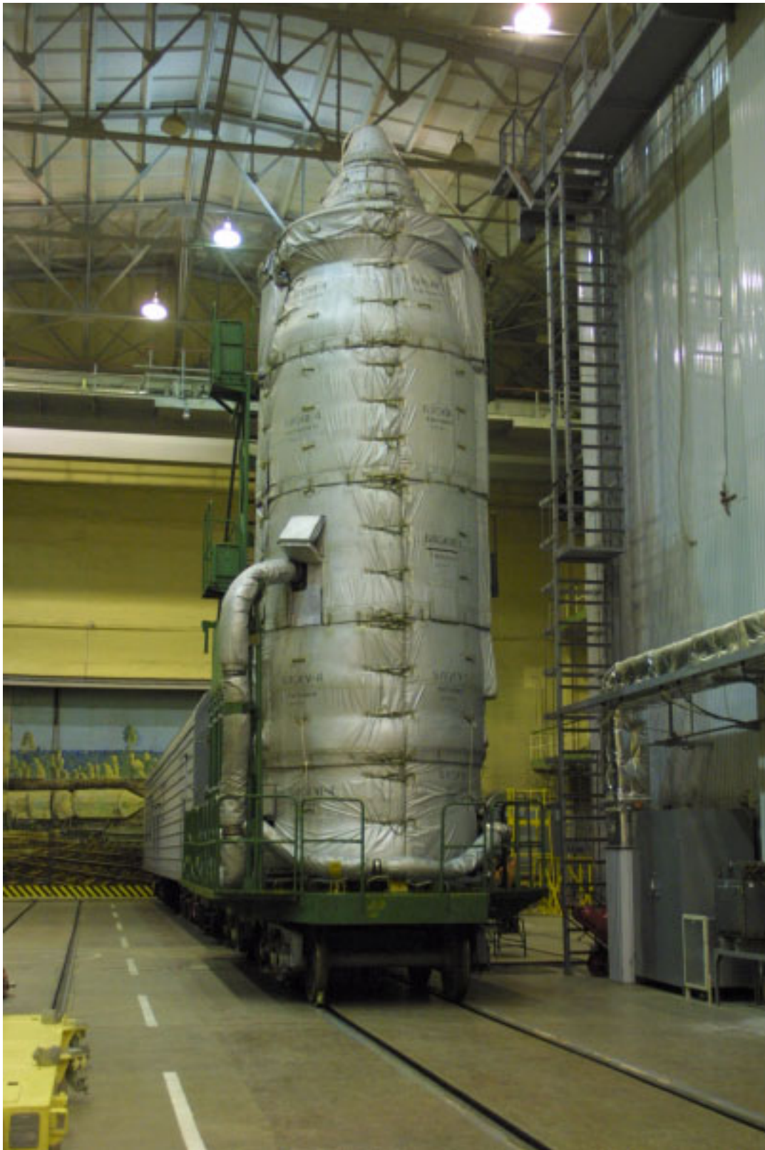
Figure 1-18: Fitting of Thermal Cover on Upper Composite Prior to Transfer to the Launch Pad
