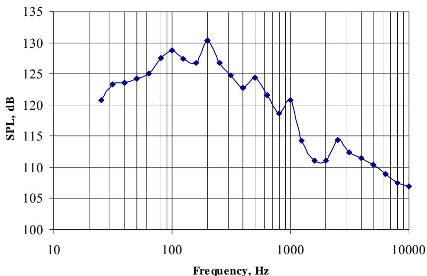
Figure 5-4: Acoustic Noise under the Rockot Payload Fairing
