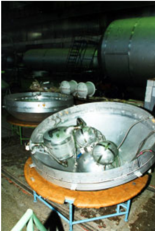
Figure 1-24: Close-up of the Breeze-KM Restartable Upper Stage in the Khrunichev Production Hall
