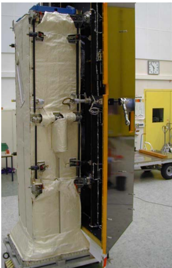
Figure 4-20: Side-mounted Multiple Satellite Dispenser System for Two Spacecraft (Note: only one spacecraft shown in this photo)
