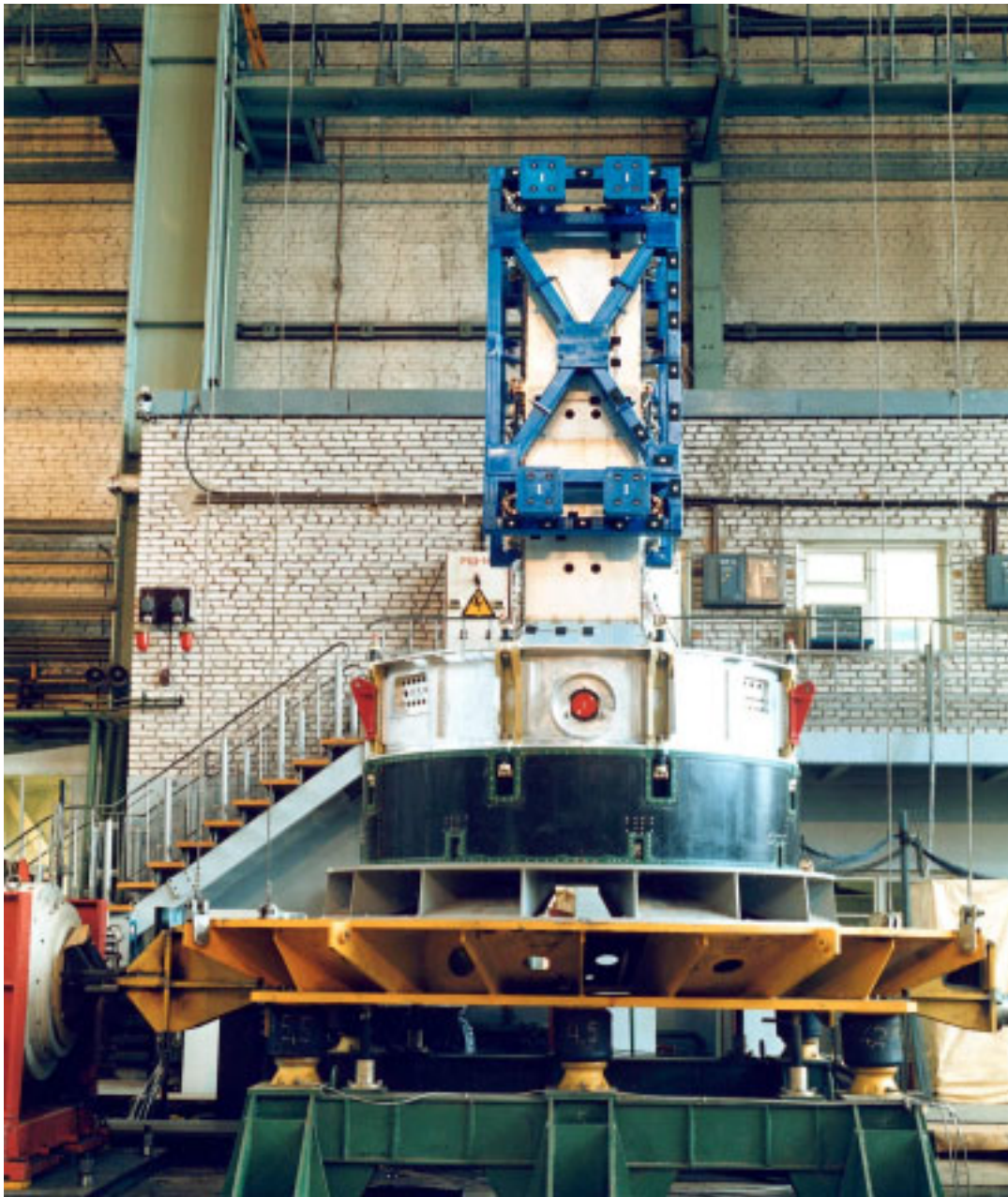
Figure 1-30: Typical Vibration Tests of a Breeze-KM Upper Stage with Spacecraft Mass-Frequency Simulators (GRACE)
