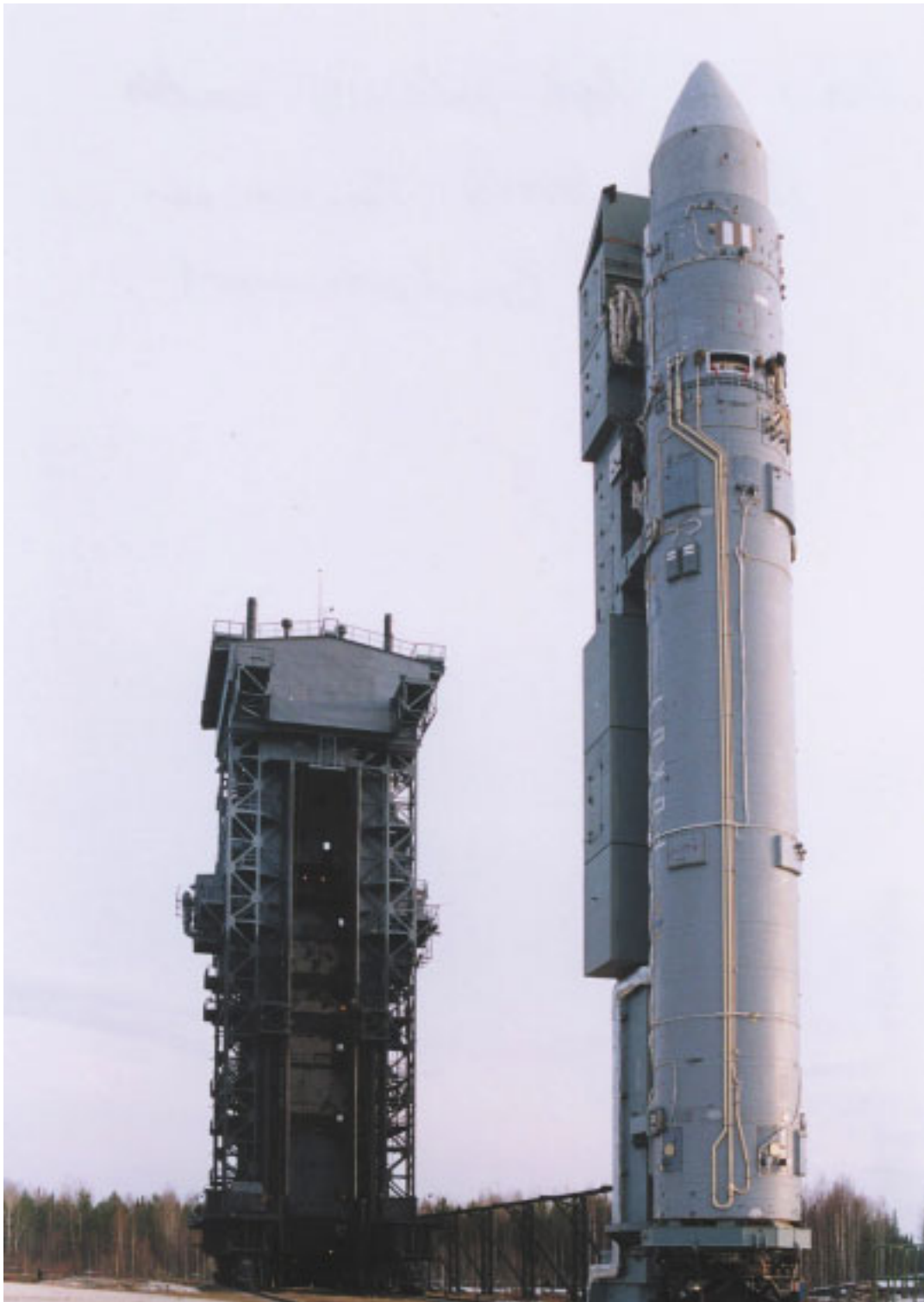
Figure 1-23: Rockot Launch Vehicle Ready for Launch with Mobile Tower Rolled Back
