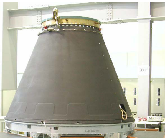
Figure 4-16: Payload Adapter for the CASA CRSS 937 SRF Clamp Band
