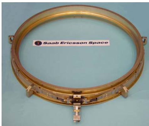
Figure 4-6: Saab Ericsson Space PAS 937S adapter, S/C aft ring and low shock separation system
